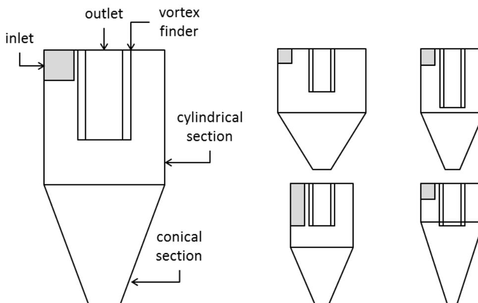
Figure 1: Typical cyclone layout and examples of design modifications\*
