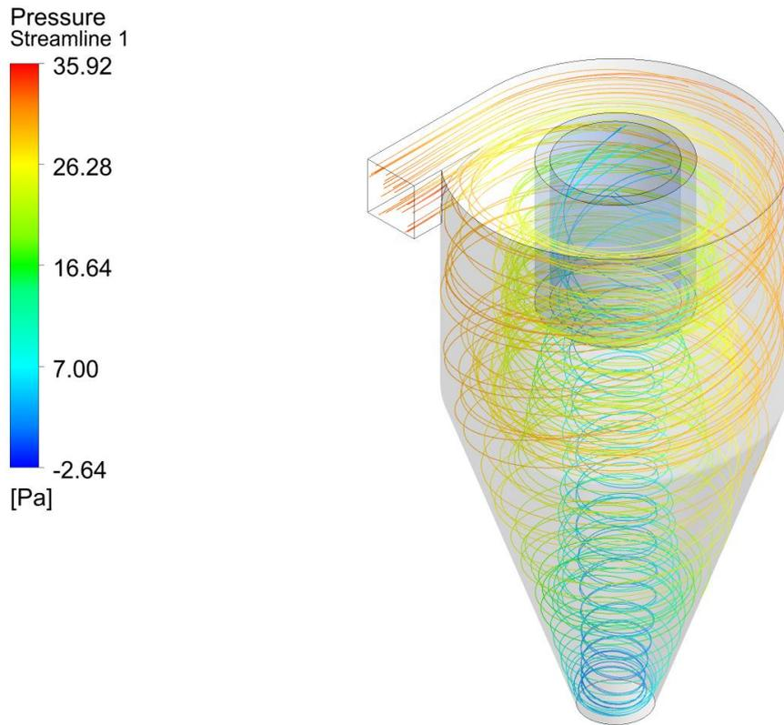
Figure 2: Flow of the gas phase in a cyclone (colored by pressure)
