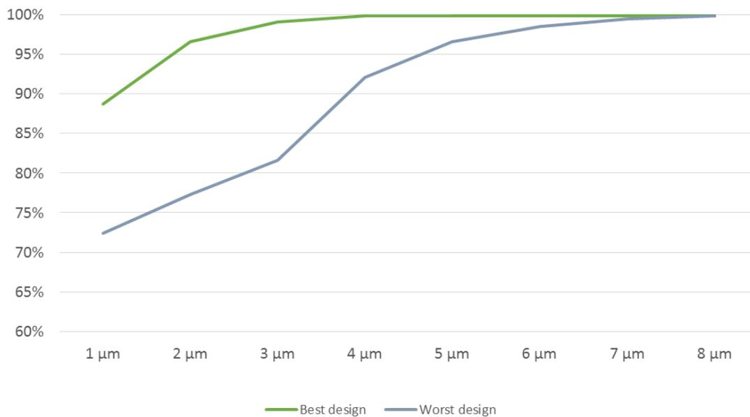
Figure 3: Cyclone collection efficiency as a function of particle size for two different set-ups
