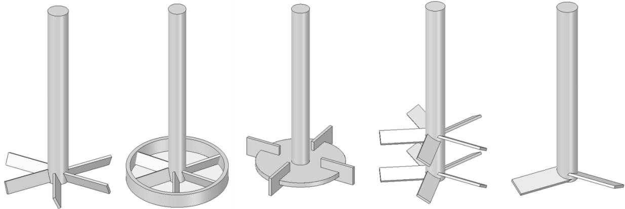
Figure 1: Examples of typical stirrer layouts and design modifications\*
