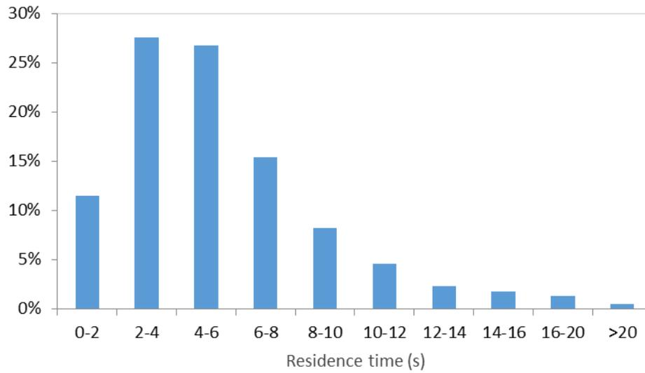
Figure 4: Residence time distribution of injected gas bubbles
