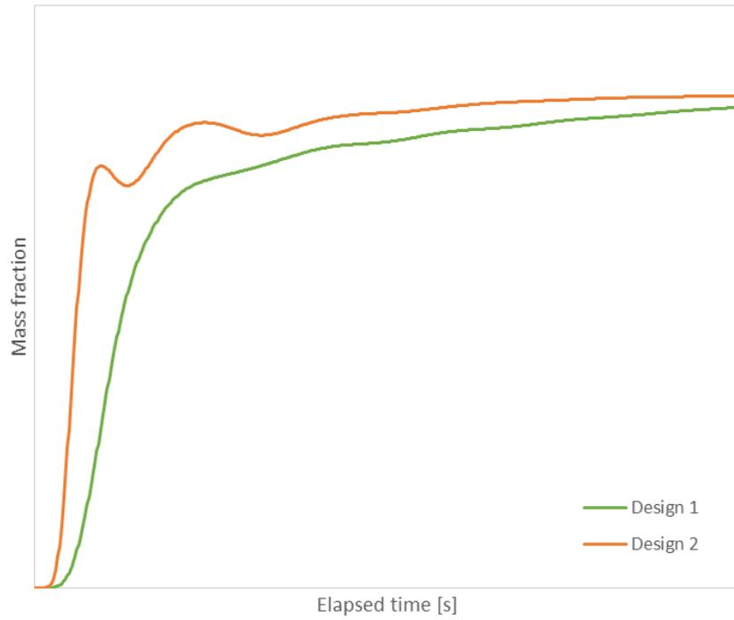
Figure 2: Tracer concentration as a function of time after addition, to assess mixing times for two different set-ups
