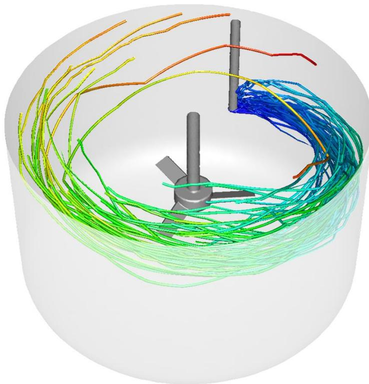
Figure 3: Flow of injected gas in a lead refining kettle
